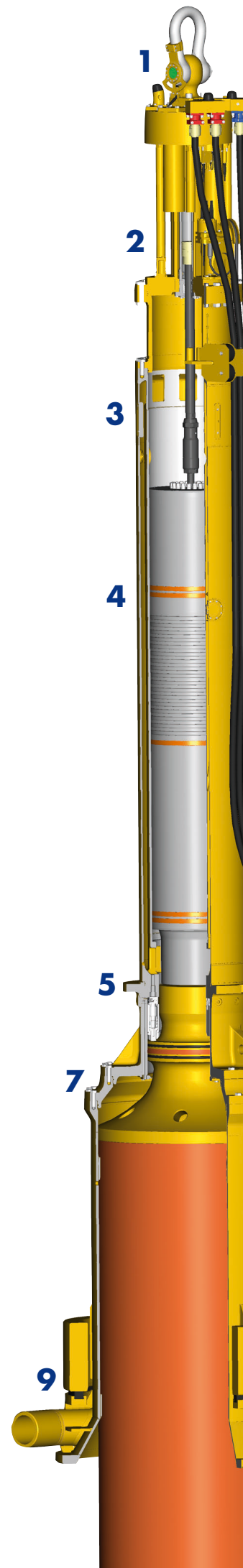
4 Ram position control-stroke height and energy - via proximity switches
